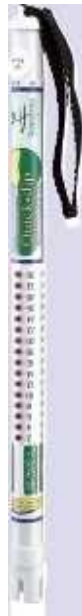
ABOVE RIGHT: Constant readout, temperature-compensated EC/ppm meters with a probe immersed in the nutrient tank provide round-the-clock intelligence.
