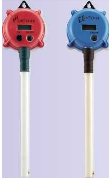
ABOVE LEFT: The probe of this meter is submerged in the nutrient solution to monitor pH 24 hours a day.
